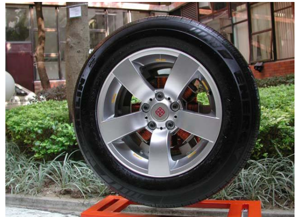
Fig 9: In-wheel motor with the cover open.
