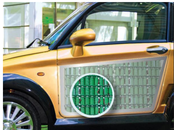
Fig 5: Distributed energy storage concept for vehicles.
